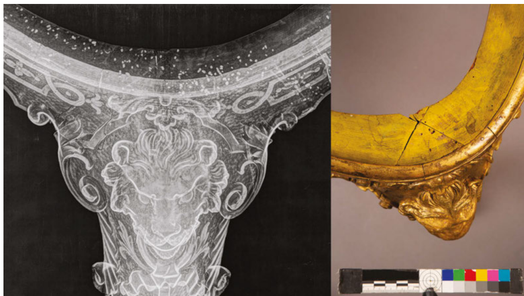
X-ray photograph of a front corner leg and adjacent seat rails showing that the rails and leg are joined without tenons. © Metropolitan Museum of Art, 24.136.1
