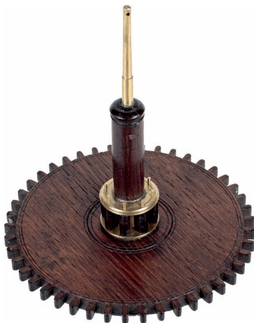
Fig 4. A striking train wheel, oak, lignum vitae and brass. The grain of the oak of the wheel teeth are aligned radially, as with all the wooden wheels. Photograph by Jeff Darken
