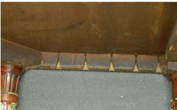
Fig. 4 Detail showing the bottom of the carcass dovetailed into the sides of Fiedler commode. By kind permission of the Trustees of the Wallace Collection
